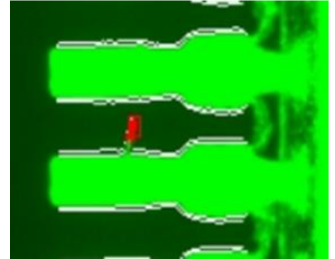
Burr Detection (down to 7\mu\text{m} defect size)
