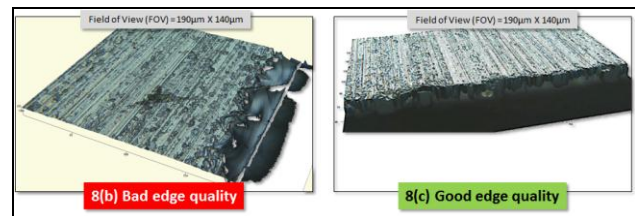
Fig. 8(b) and 8(c). Bad and good wafer edge.
