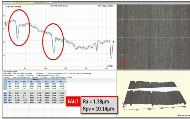
Fig. 5(b). Bad wafer quality after slicing
