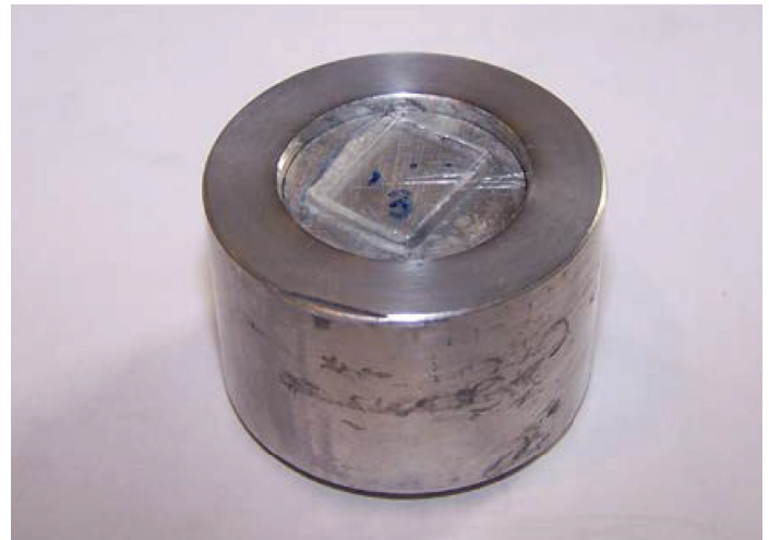
Figure 1. Fixed mouse lung cells mounted in a fluid puck for scanning and testing with the Nano Indenter G200 system.
