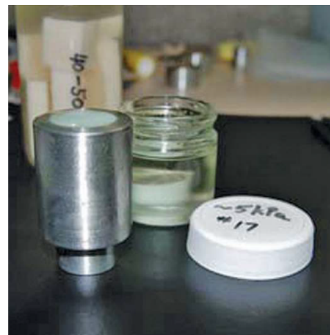
Figure 2. Phantom tissue as mounted for testing in fluid.
